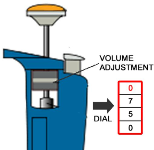
Micropipette volume setting. Adapted from "Gilson Schematic" by Squidonius.
